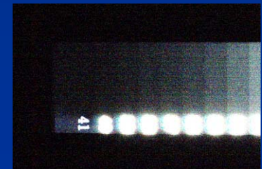
Extremely exaggerated section of digital image shows resolution of all 41 steps PLUS opaque surround!
