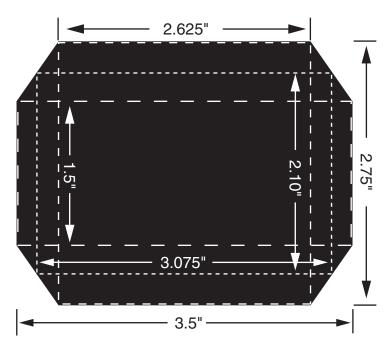
NOTE: The full octagonal area shown will be captured by the Better Light scan back. Exact shape of final image can be controlled by the cropping and resolution settings in the Better Light ViewFinder™ Software.
