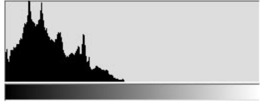
Histogram of an underexposed scene.
